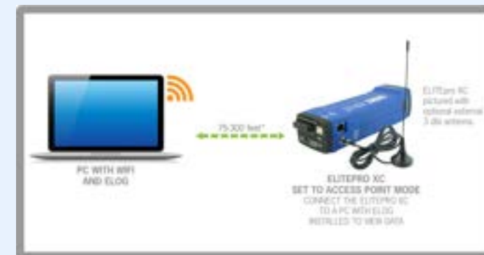
Access Point mode sets the ELITEpro XC as an access point. View real-time data on a wi-fi-enabled laptop running ELOG software.
